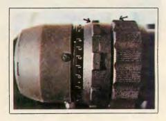
Both reticle and telescope focusing on this passive unit are controlled by manipulation of radical bands on telescope body itself. Makes for streamlined profile that doesn't catch on vegetation, web gear, etc.
